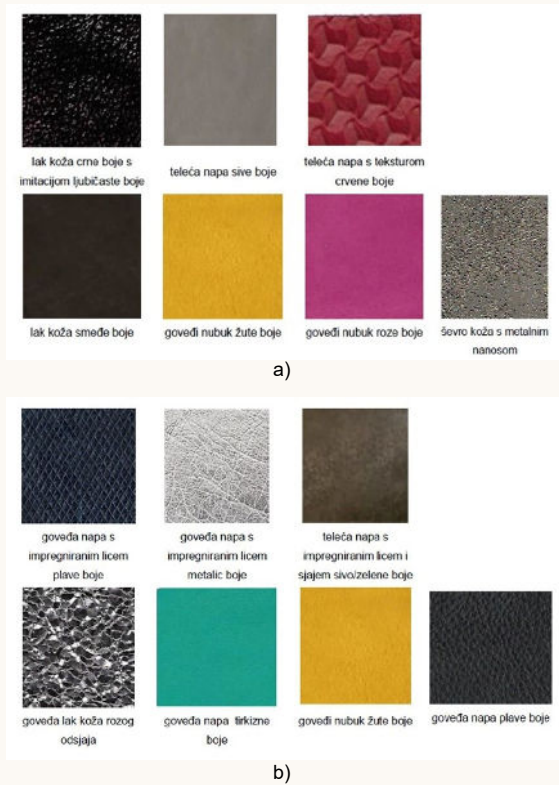
Figure 4. Leather samples: a) for sneaker and backpack No. 1 and b) for ankle boot and backpack No. 2 [8].
