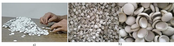
Fig. 18 The smallest leather applications: a) perforated circular pieces of leather, b) finished look of leather circles [3]
