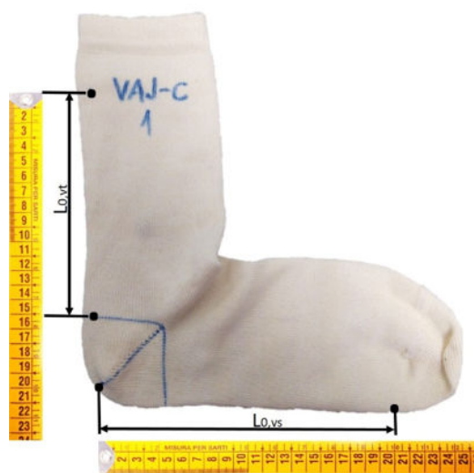
Fig. 4 Sample marking for measuring geometrical parameters of the unstretched sock
