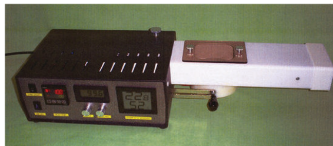
Figure 1: PERMETEST - device for non-destructive determination of water vapour and thermal resistance, by Sensora Instruments [17]
